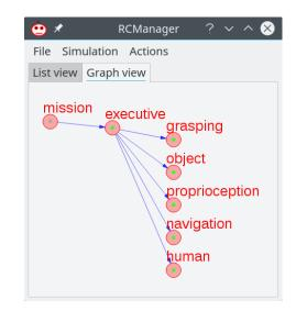
Fig. 4: Deployment network of the high level components used in these examples of use.
